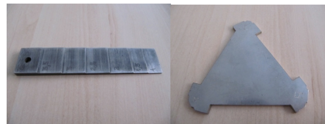
Figure 2 – Templates for visual inspection of welding
